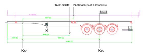
Following load analysis aims to get as much Payload weight as possible whilst not overloading allowed 24/15 tonne bogie & kingpins loads respectively. In doing this the overall combination of weights exceeds the maximum 44 tonnes. To maximise the axle loadings, and operational combination weight of 46.245 tonne is required. This allows for a payload of 30,976 kgs including the container self-weight. Based on a container weight of 4790 Kgs, this would leave a goods payload of 26,181 kgs.
