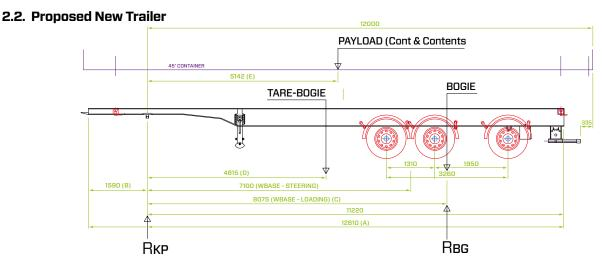
Following load analysis defines the operational weight at 48 tonne, with the trailer geometry being customised within this figure to achieve a 27 tonne bogie, as defined in current UK C&U, whilst not exceeding 16 tonne on the kingpin in order that truck loadings also, will not fall outside existing C&U regulations.
