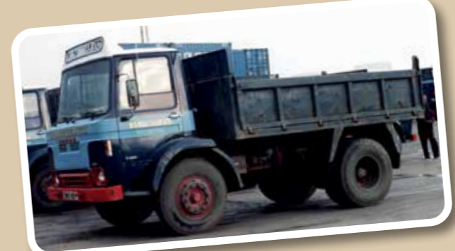
Michael's first motor at Malcolm's was to be a four wheel Dodge Commando just like this one. There were about 10 of these in service at Castlebank Street and they were good for a 10 tonne payload.
