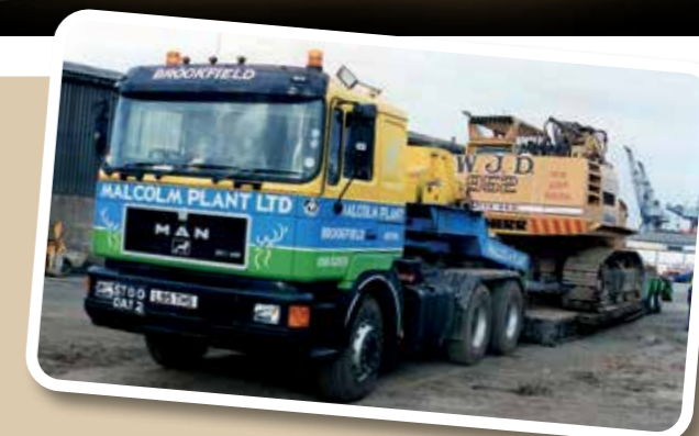
STGO Cat 2 allowed for operations of up to 80 tonnes gross. Michael recalls that the outfit is unloading a customer's machine at Castlebank Street depot where it would be kept until required for its next job.
