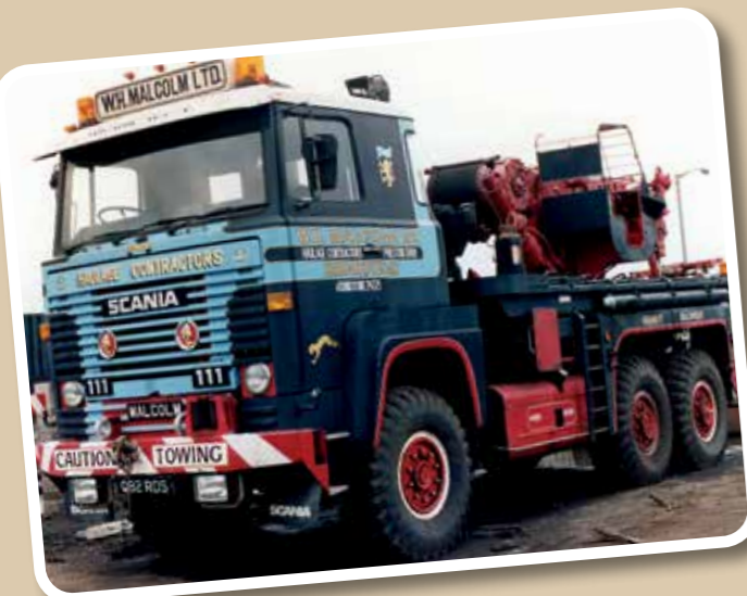
Malcolm vehicles don't come much more distinctive than 'The Mongrel' which originally started life as a Rolls-Royce (petrol) powered Leyland Martian 6x6. Later fitted with a Scania cab and engine, it's recalled for its phenomenal winching ability.
